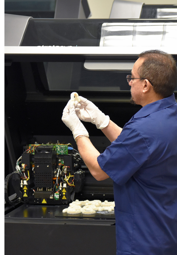
The Stratasys J700 Dental 3D Printer is capable of producing 50-60 arches per print tray.
