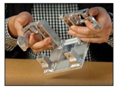
The assembly fixture on the left is made up of multiple parts that are welded and pinned together.
