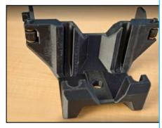
In contrast, the 3D printed fixture on the right serves the same purpose but is made up of fewer parts and can be printed in a single print operation.
